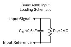
The Sonic 4000 RF active probe uses a PMK custom high speed FET input amplifier with active cladding wave compensation to provide a superior high frequency response as well as a low noise and low distortion to accurately measure the customer signals. The output signal of the probe has no DC component, so it can be connected to DC sensitive measurement equipment.
