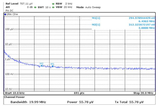
Low frequency noise:  $10 \, \text{kHz} - 20 \, \text{MHz}$ :  $56 \, \mu V_{rms}$
